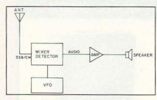
Figure 1. Diagram of the basic direct conversion receiver.
